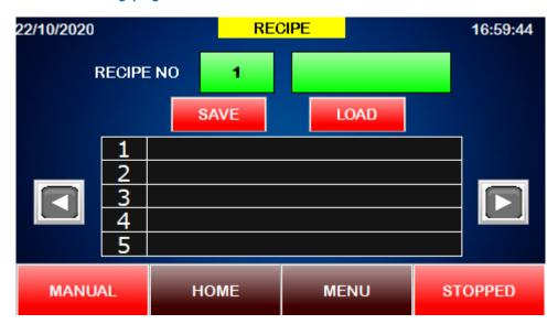
• This page is used to save and load the different filling parameters.
