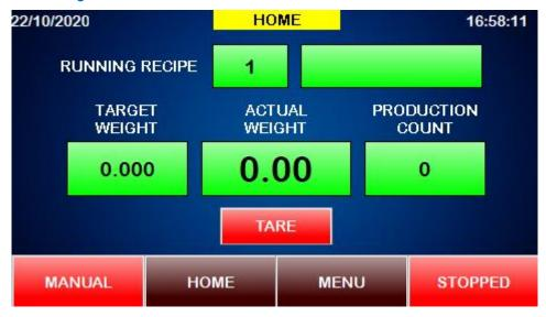
• This page displays the current weight, target weight and production count, and currently running recipe.
