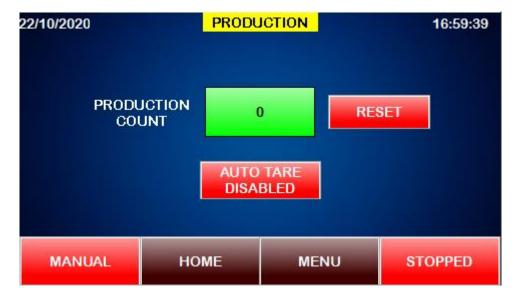
This page is used to reset the PRODUCTION COUNT, and Enable/Disable the AUTO TARE Functionality.
