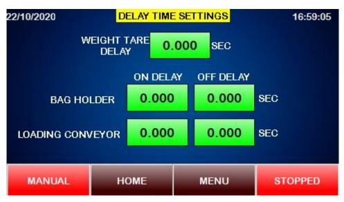
This page is used to set the Timing control for each outputs like BAG HOLDER, LOADING CONVEYOR, TARE DELAY TIME.
