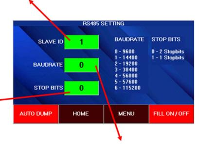
The Stop Bits for RS485 can be written. The Last Changed Stop Bits will be retained until next change.
