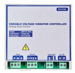
Key advantage of ECVC20 is that, it comes with mains voltage compensation algorithm, which keeps the vibration same even when the supply voltage increases or decreases. Hence the material flow remains constant even though supply voltage varies, thereby increasing the system accuracy.
